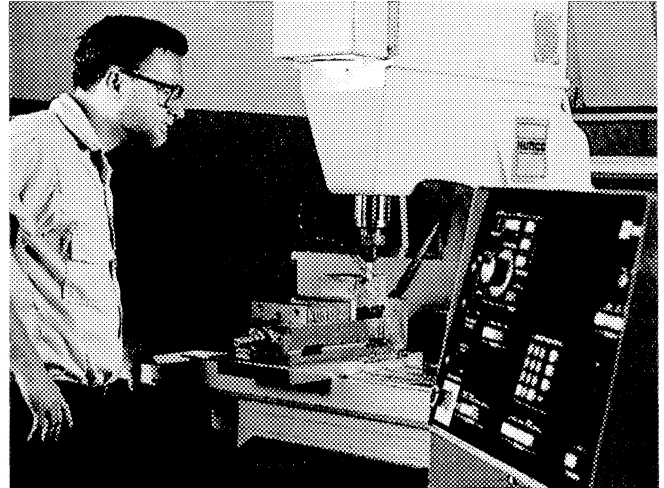
FIGURE 14.18 Part Being Machined on a Vertical Mill
